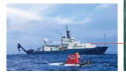
The sub Alvin stavs buoyant with the help of syntactic foam, now rated to go four miles underwater. The foam is composed of billions of glass air bubbles the size of powdered sugar, encased in resin.
